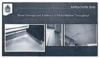
There is also water damage and evidence of mold and mildew throughout the building. These are just a few of the pictures. The entire envelope of the building is has penetrations and you can actually see the outside from the inside in multiple areas.
